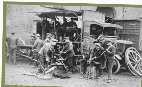
Troops of the Army Ordnance Corps re-assembling and repairing guns at a mobile workshop in France, 1918 © IWM (Q 347)
